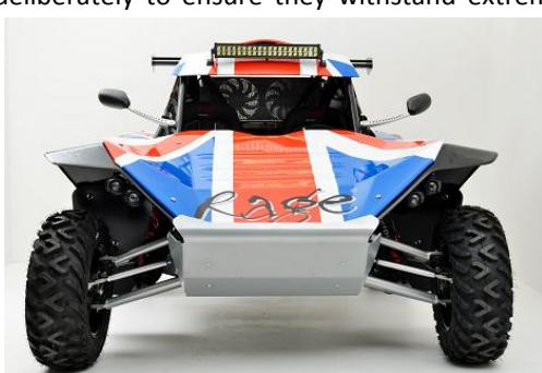
We use a double wishbone configuration all round with anti dive, when braking hard, built into the front. The design also limits any camber, caster, bump steer and high speed stability problems inherent with other alternatives such as trailing arm, which can be problematic when large amounts of suspension travel are available. The Rage suspension travel is front 12.5" and rear 13.5"
